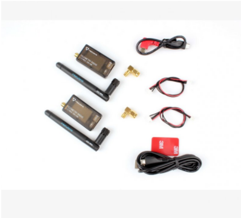
Figure 6: 433MHz Holybro telemetry radio set
