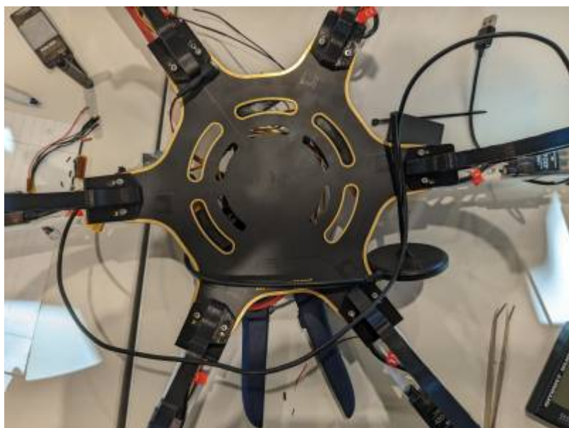
Figure 8.2 Adding 6 landing gear to 6 base frame
