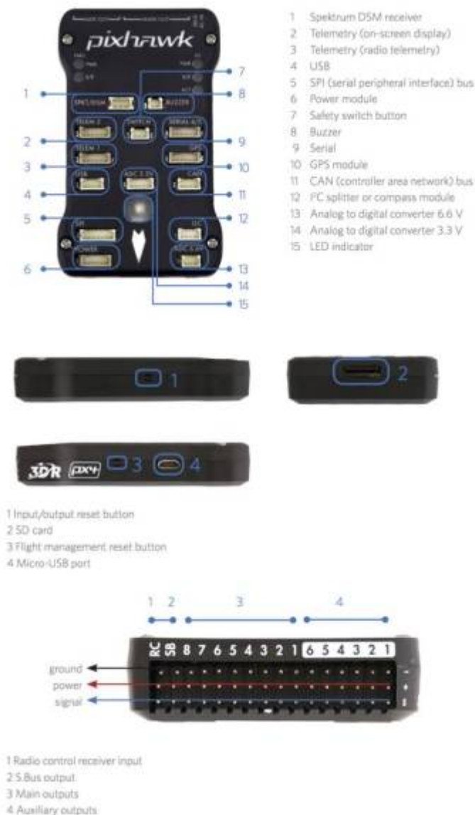
Figure 7.1 Diagram of PixHawk 2.4.8
