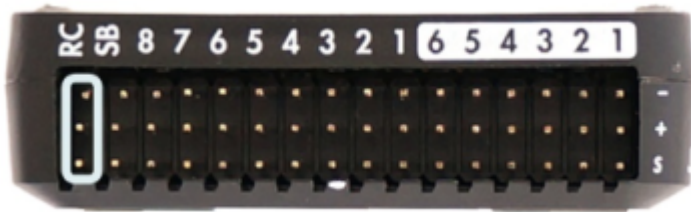
Figure 7.6.1 Connecting radio control to RC port in flight controller
