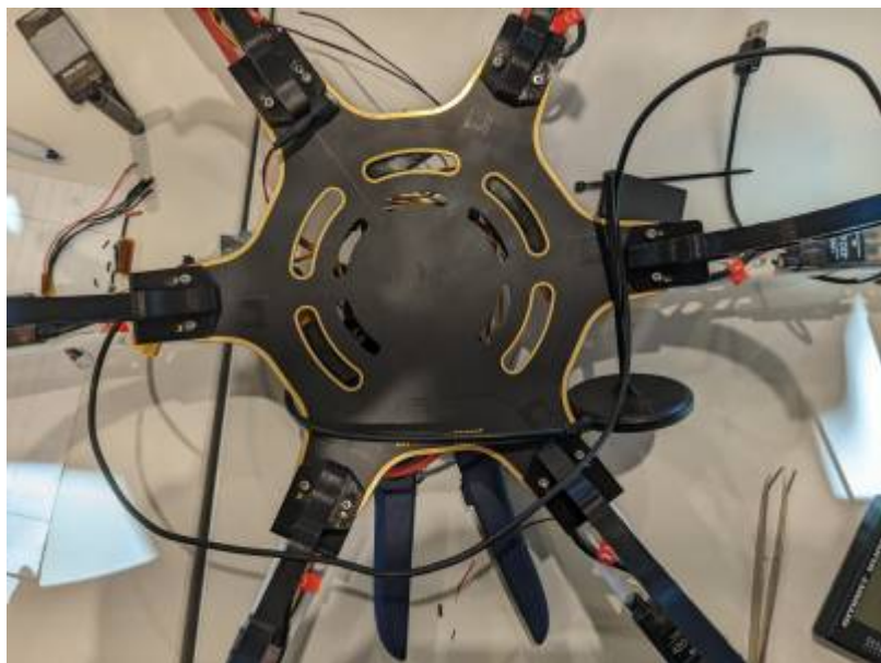
Figure 8.2 Adding 6 landing gear to 6 base frame
