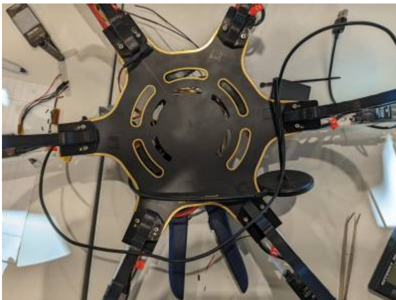
Figure 8.2 Adding 6 landing gear to 6 base frame
