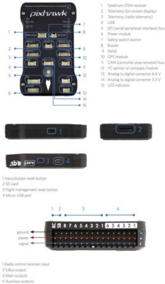
Figure 7.1 Diagram of PixHawk 2.4.8
