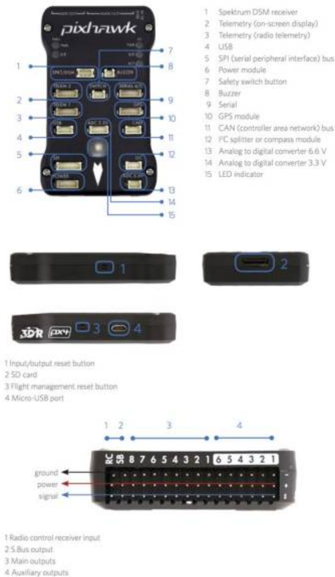
Figure 23 Diagram of PixHawk 2.4.8
