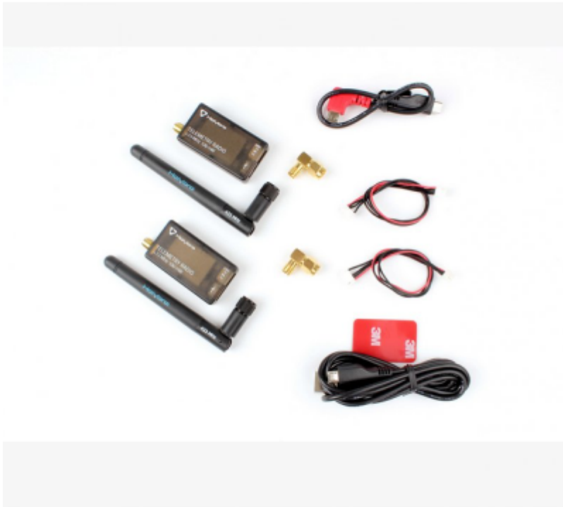
Figure 6: 433MHz Holybro telemetry radio set
