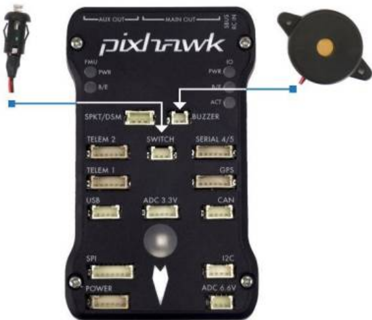
Figure 25 Safety switch and buzzer location and connection
