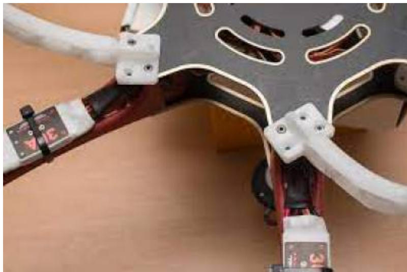
Figure 21 using zip ties for mounting ESCs to the arm
