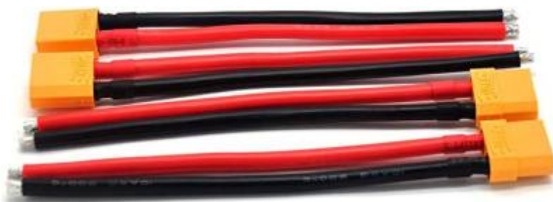
Figure 18 Soldering wires to XT60 connector
