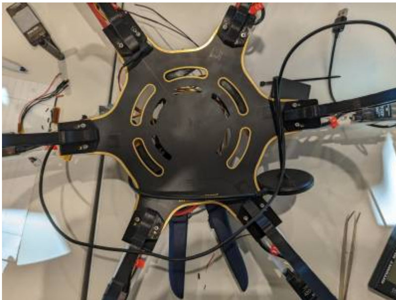
Figure 34 Adding 6 landing gear to 6 base frame
