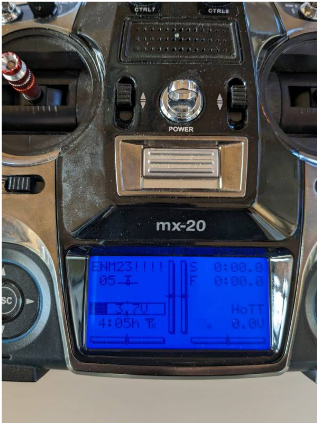
Figure 38: Graupner transmitter confirming receiver binding
