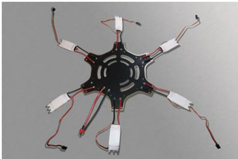
Figure 17 basic skeleton with all ESCs and power supply cable attached
