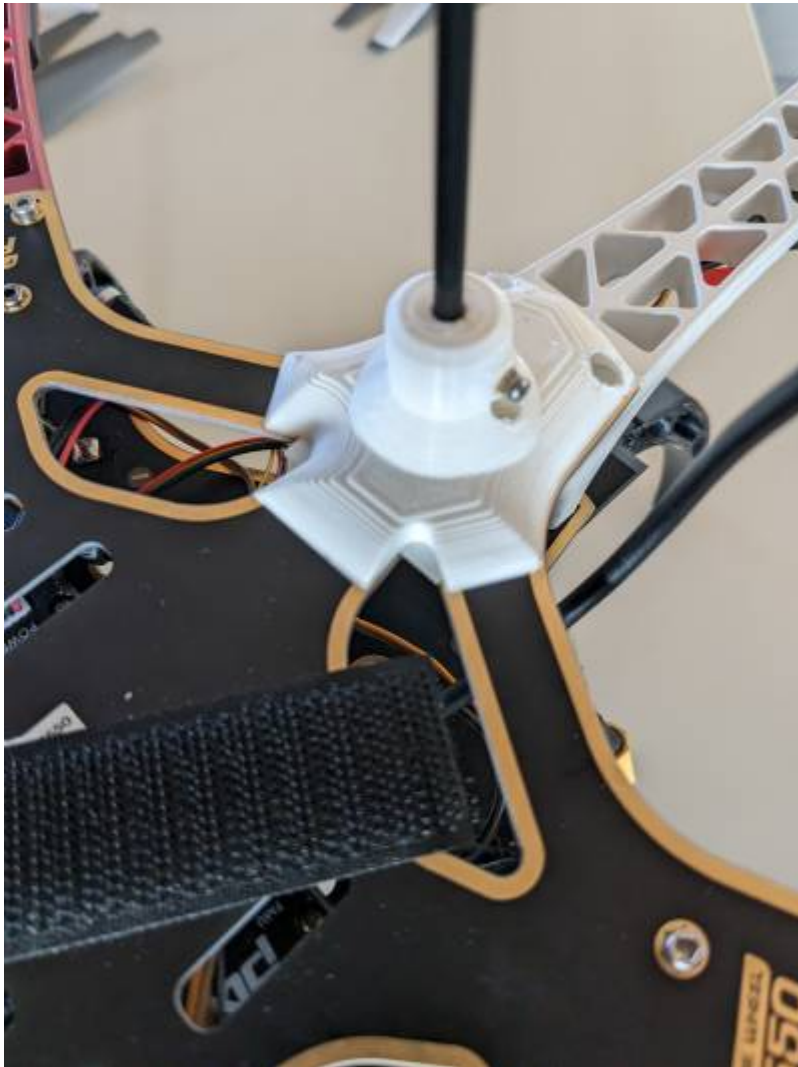
Figure 35 Mounting GPS unit on top frame
