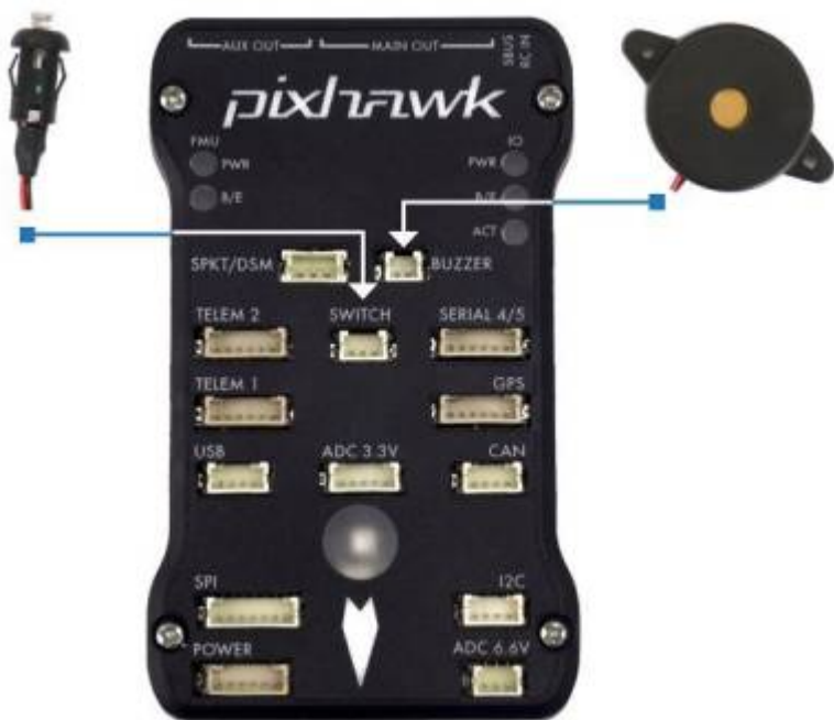
Figure 25 Safety switch and buzzer location and connection
