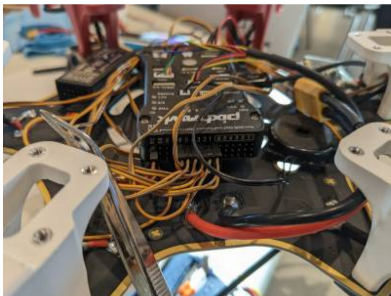
Figure 31 Connecting ESCs to the flight controller
