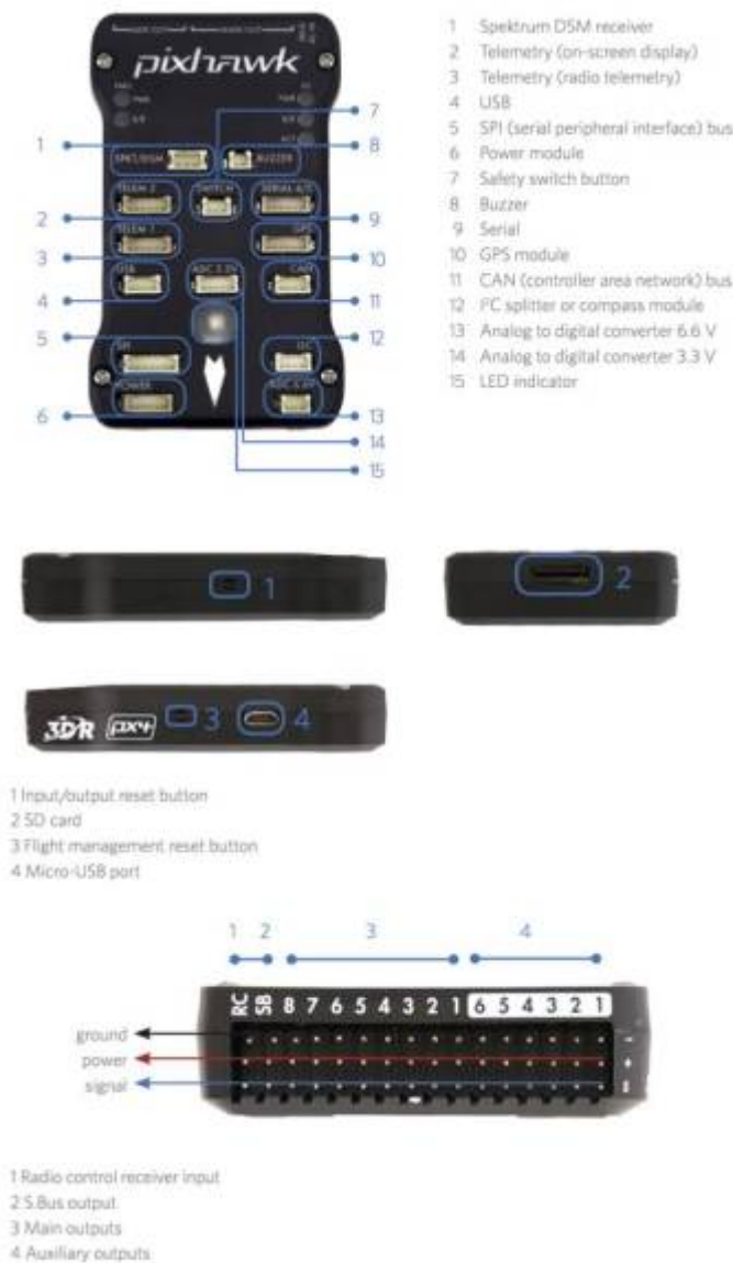
Figure 23 Diagram of PixHawk 2.4.8
