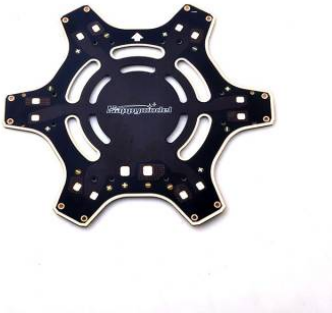
Figure 16 Connections with positive and negative symbols on base frame
