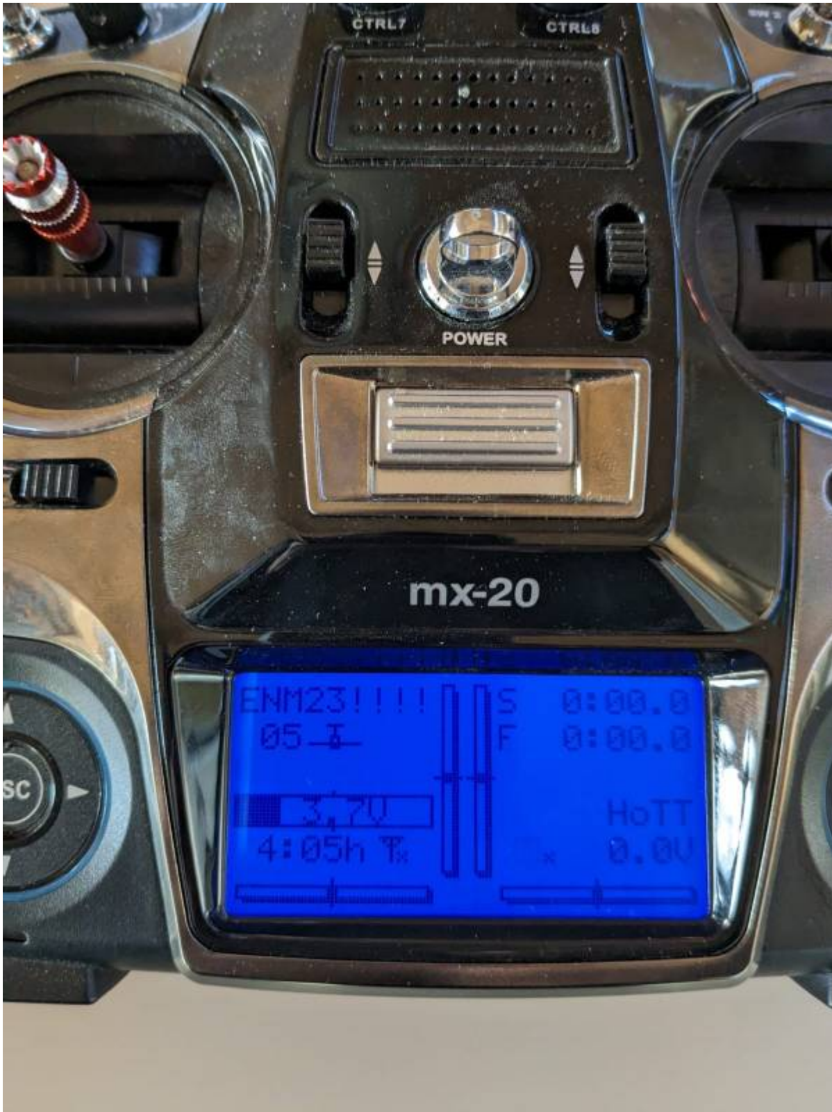
Figure 38: Graupner transmitter confirming receiver binding
