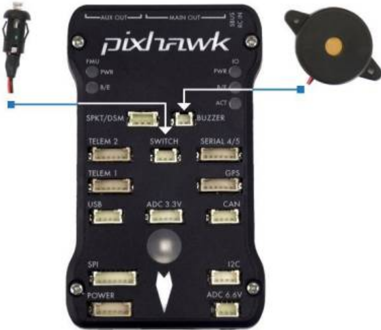
Figure 25 Safety switch and buzzer location and connection
