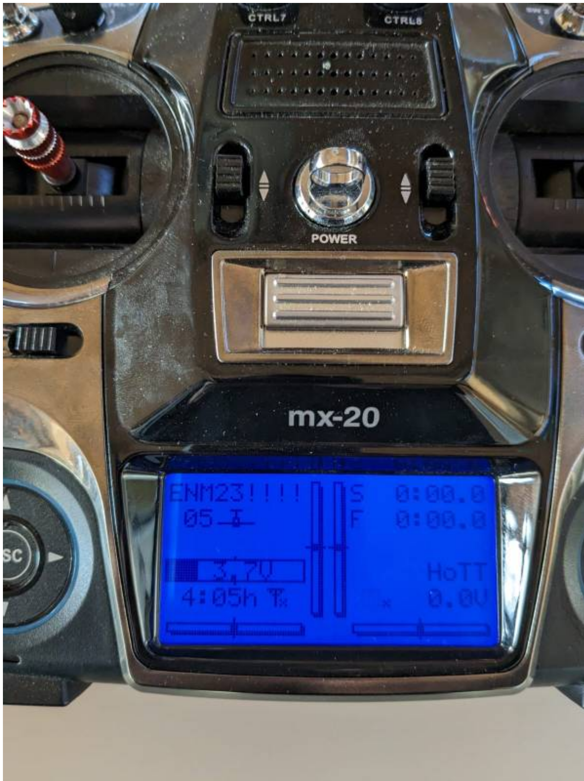
Figure 38: Graupner transmitter confirming receiver binding
