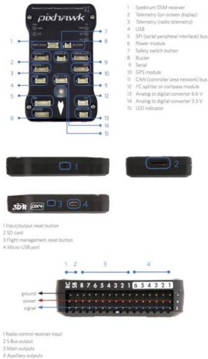
Figure 23 Diagram of PixHawk 2.4.8
