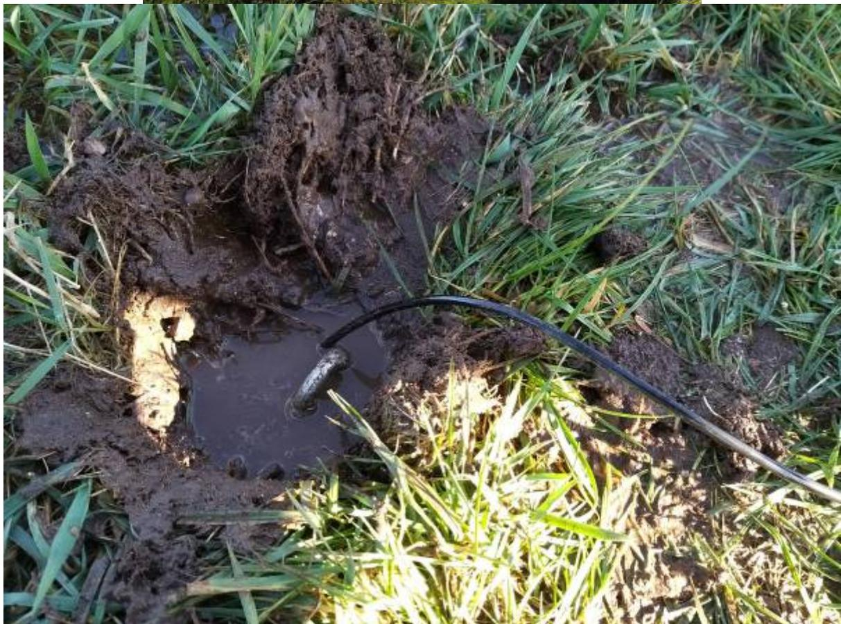
Because this particular field is used for cows in the summer, the wire needed to be buried underground. In the future the sensor node should be moved higher.
