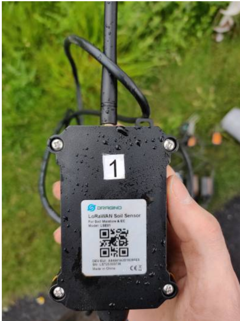
Waterproof housing of the LoRa node.
