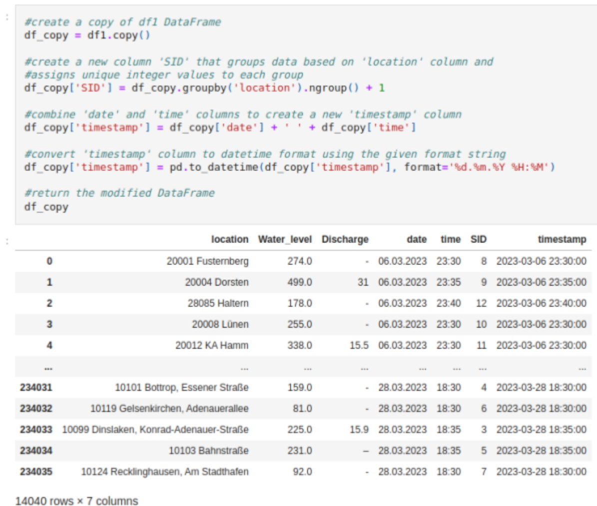
Figure 14. Adding SID and timestamp
