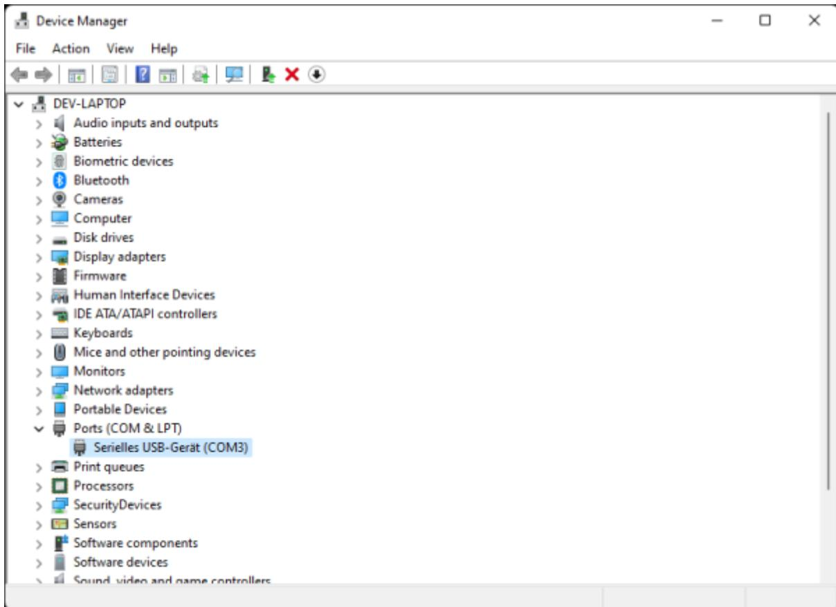
Double click each USB Serial Device entry so you can check its properties. Go to the **Details** tab, in property select **Hardware Ids**. If you see **VID 0955** and **PID 7020**, that USB Serial Device for your Jetson developer kit. Note the COM port name (COM3 in this example) for later use.
