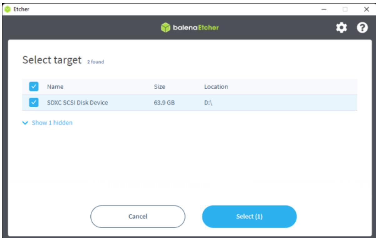
Click **Flash!** It will take Etcher about **10 minutes** to write and validate the image if your microSD card is connected via USB3.
