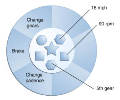
By attributing state (current speed, current pedal cadence, and current gear) and providing methods for changing that state, the object remains in control of how the outside world is allowed to use it. For example, if the bicycle only has 6 gears, a method to change gears could reject any value that is less than 1 or greater than 6.
