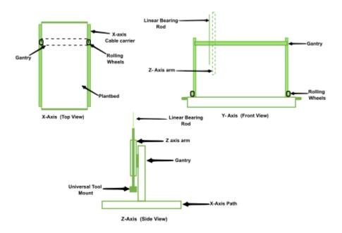
Fig - 4.1 Line Diagram structure of Farmbot
