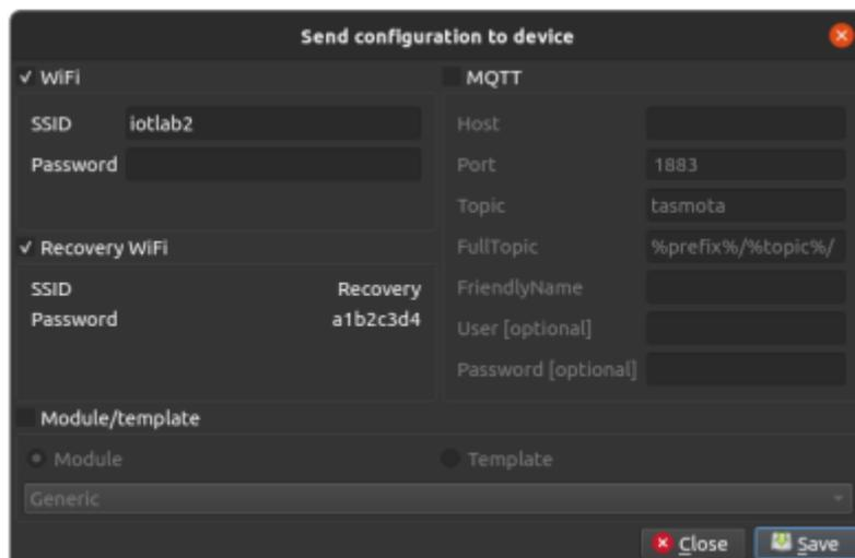
We are going to use them to set the WiFi credentials. For later use the **Recovery WiFi**-Option could be helpful. When the ESP8266 can not connect to the configured WiFi, it will open up a WiFi-Hotspot. You can then connect to it and make configuration changes. We will not use the other options in the **Send config** window.
