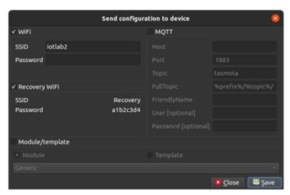
We are going to use them to set the WiFi credentials. For later use the Recovery WiFi-Option could be helpful. When the ESP8266 can not connect to the configured WiFi, it will open up a WiFi-Hotspot. You can then connect to it and make configuration changes. We will not use the other options in the Send config window.
