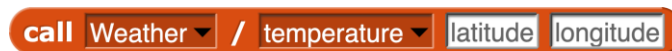
Figure 1. The temperature RPC of the Weather service. Selecting a service from the first pull-down menu populates the second with the available RPCs. Selecting an RPC reconfigures the call block to present slots for the required input arguments and provide their names as a hint.
