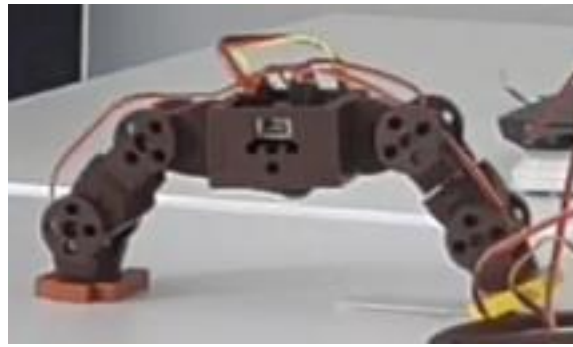
Figure 8. Worm with 4-degrees of freedom, the first robot we have built from the modular components
