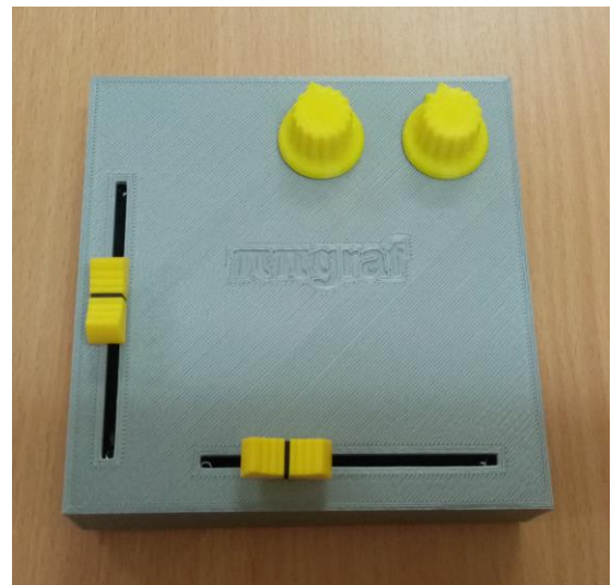
Figure 1. ππgraf as designed in OpenSCAD and produced on a 3D printer.
